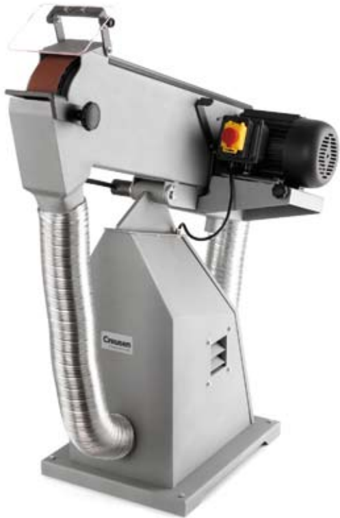
BS 975A/HD 3~ with integrated dust extraction Voltage: 400/230V 3~ 50-60Hz art. 007821 Power: 4 kW Speed: 2800-3400 rpm Belt size l x w: 2000 x 75 mm
