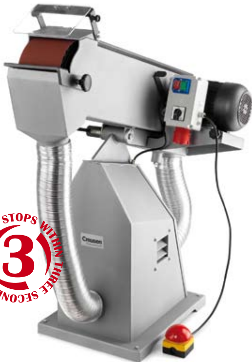
BS 9150A/HD-B-2n 3~ with integrated dust extraction, brake and 2-speed motor Voltage: 400/230V 3~ 50-60Hz art. 007848-B-2n Power: 4 kW Speed: 2800-3400/1400-1700 rpm Belt size l x w: 2000 x 150 mm
