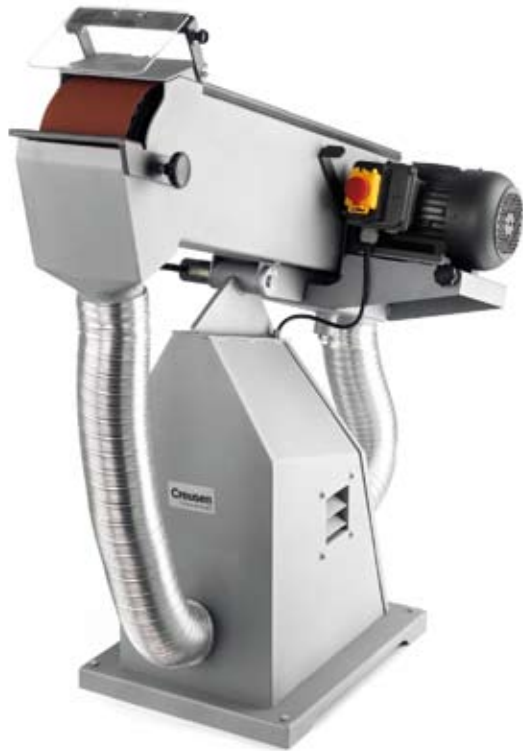
BS 9150A/HD 3~ with integrated dust extraction Voltage: 400/230V 3~ 50-60Hz art. 007843 Power: 4 kW Speed: 2800-3400 rpm Belt size l x w: 2000 x 150 mm
