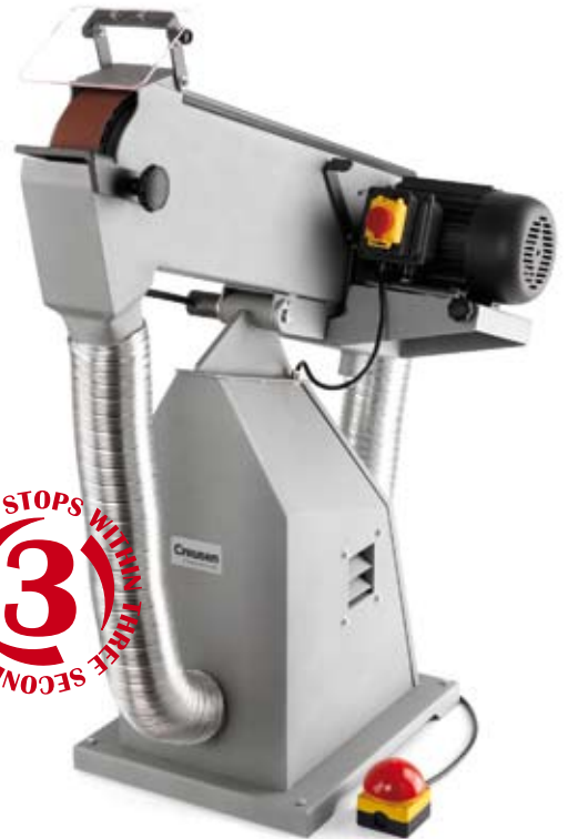
BS 975A/HD-B 3~ with integrated dust extraction and brake Voltage: 400/230V 3~ 50-60Hz art. 007825-B Power: 4 kW Speed: 2800-3400 rpm Belt size l x w: 2000 x 75 mm
