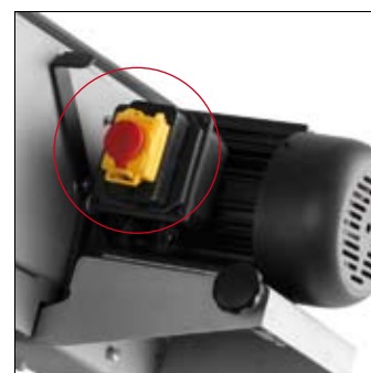
Switch with no-volt release and emergency stop
