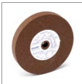
Grinding wheel normal corundum ø 150 x 20 x 15 mm, grit 80 art. 700128
